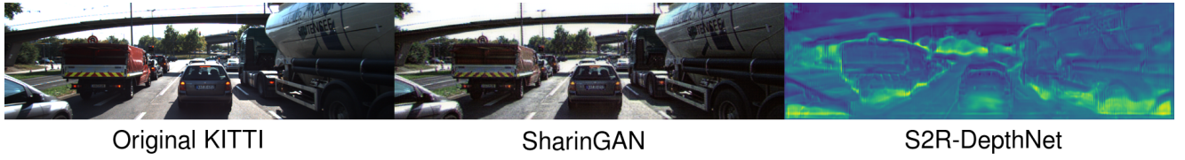
Fig. 9 Transfer of KITTI images to the intermediate shared domain employed by SharinGAN (PNVR et al., 2020) and S2R-DepthNet (Chen et al., 2021). The original single-channel S2R-DepthNet images are mapped to RGB using a colormap and logarithmic mapping.
